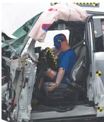
The extended cab is a different story. Intruding structure seriously compromised the driver’s survival space, resulting in a poor structural rating. The toepan, parking brake and brake pedal were pushed back 10-13 inches toward the dummy, and the dashboard was jammed against its lower legs. Measures recorded on the dummy indicated there would be a moderate risk of injuries to the right thigh, lower left leg and left foot in a real-world crash of this severity.
